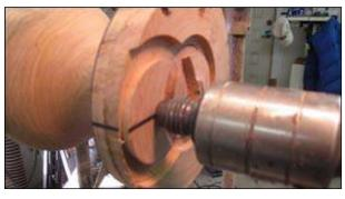
This second tenon will be used to form the neck of the vase. It might be easier to start the recess with a small gouge and then finish it with a bedan or parting tool.
