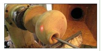
Use smaller tools. I highly suggest using a captured hollowing bar because you will be less likely to get a catch. You will be very close to the side of the vessel on one side but not on the other. Make sure you keep this in mind, or you will create a second opening in the vessel.
