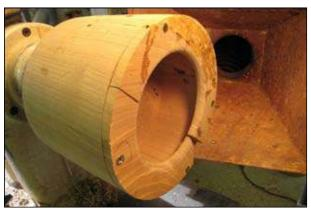
This doesn't work for all vessel shapes. Put the top of the vessel in/on the drum chuck and bring up the tailstock for support.
