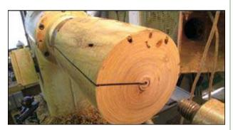
On each end, connect this line to the center point of the cylinder. Measure in from the outside edge to mark the center point for the second axis. I typically measure in 1" because that is the radius of the smallest diameter my chuck will clamp. With the best side facing up, the neck will be on the left when the finished piece is displayed. If you want the neck on the right side, the best side should be facing straight down when you draw the line.
